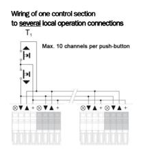
Local control with status display: Only one LED allowed. Do not link LED connections to each other.
