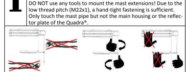
put the Quadra® with the mast extensions into the mast clamps, clos the clamps and fasten them with the screws – take care oft he orientation
