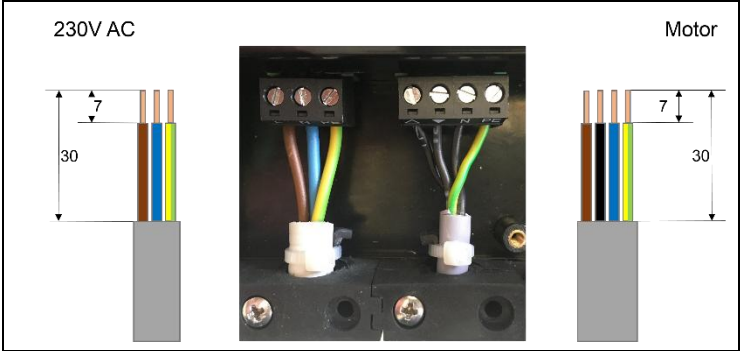
Pin assignment supply voltage / motor
